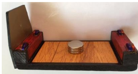
Fig. 4. Mendocino solar electric motor stator
